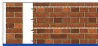
8 Creating masonry beams
