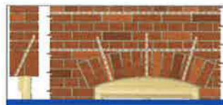
2 Repairing brick arch lintels
