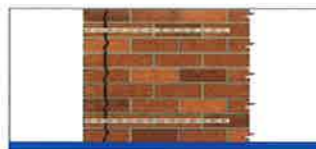
3 Repairing cracks near corners and openings
