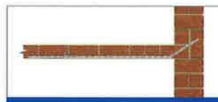
4 Reconnecting internal walls with external walls
