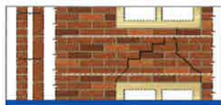
9 Repairing or creating flat arch lintels
